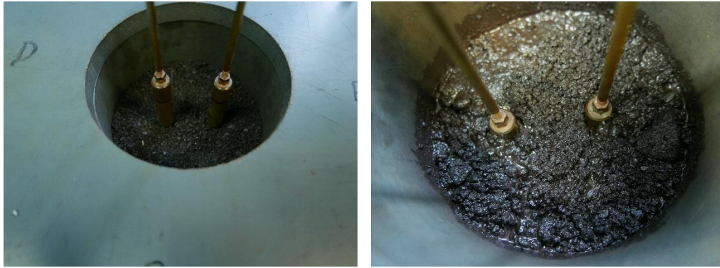
Penetration test on mill scale– before and after
