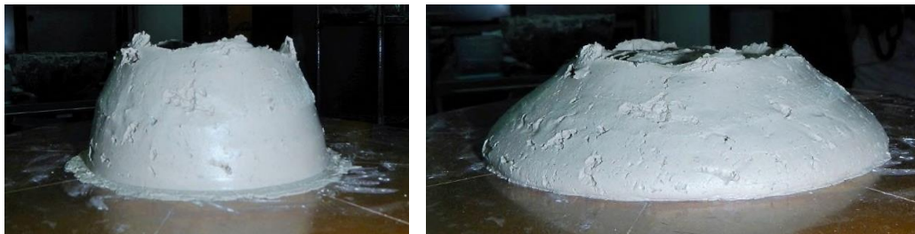
Flow table test on ball clay– before and after
